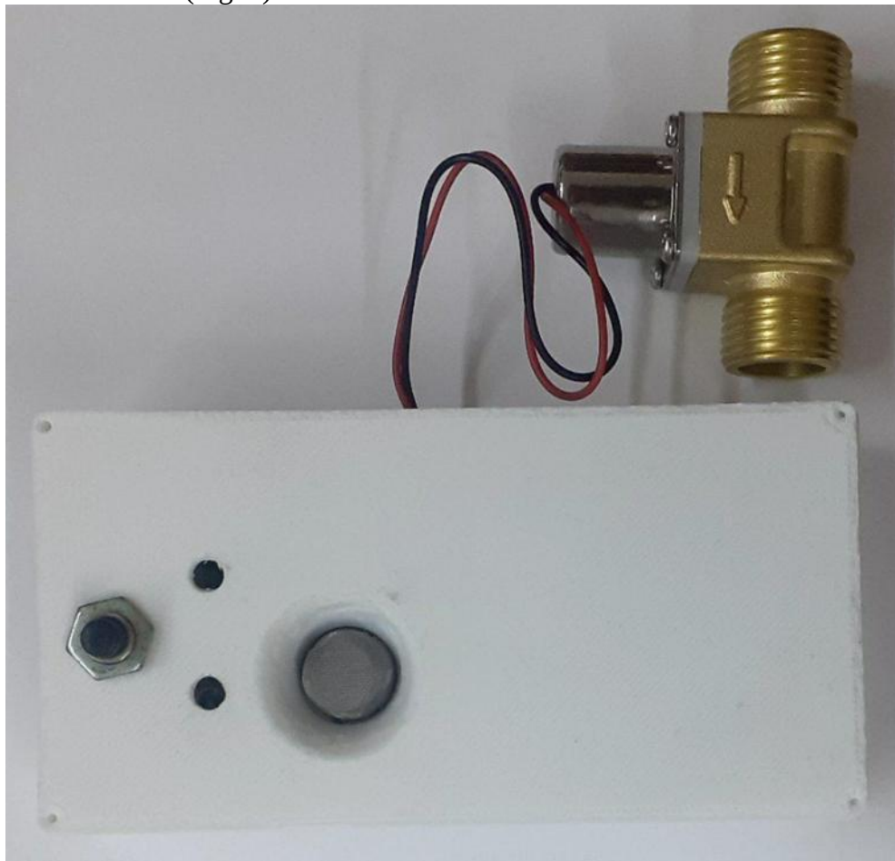
Fig. 3. Smart Gas Sensor with Shut-Off Valve
