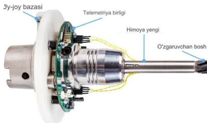
3-rasm . Sensor asboblari bilan raybalash paytida burg‘uning tekisligini o‘lchash.
