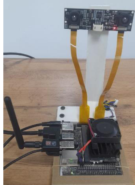
Fig. 2. Research stand based on the Nvidia Jetson Nano B01 microcomputer, equipped with an IMX219-83 stereo camera
